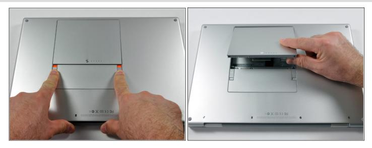
• Use your fingers to push both battery release tabs away from the battery, and lift the battery out of the computer.
